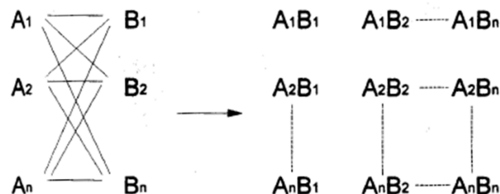
Figure 1.2. (A) In general, in a conventional synthesis one starting material A reacts with one reagent B resulting in one product AB. (B) In a combinatorial synthesis different building blocks of type A ( A_1 – A_n ) are treated simultaneously with different building blocks of type B ( B_1 – B_n ) according to combinatorial principles, i.e. each starting material A reacts separately with all reagents B resulting in a combinatorial library A_{1-n}B_{1-n} .
